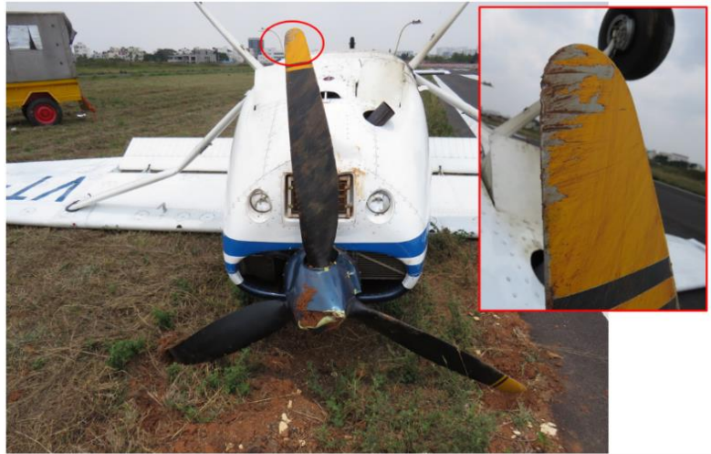
Fig 11: Propeller cone damaged (above), Nick and score marks on propeller blade (below)
