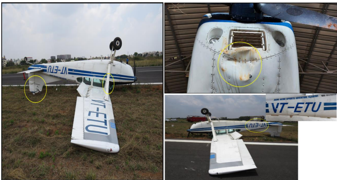
Figure 10: Clockwise - Nose Section; Dents observed on the Fuselage; Vertical Stabilizer and Rudder damaged
